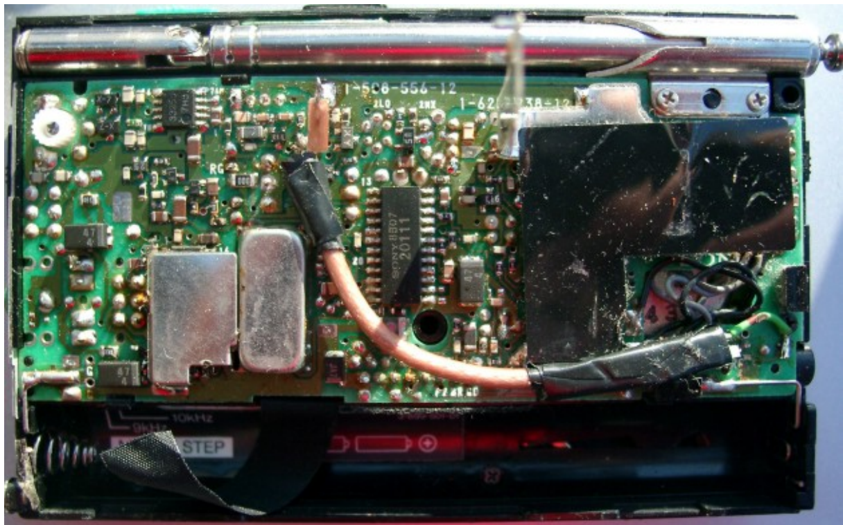
img2 : IF connection inside the ICF- SW1 (rear view, shielding removed))
