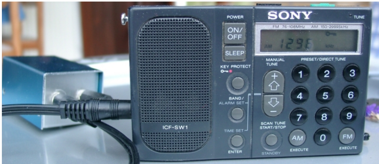
img1: Sony ICF- SW1 + drm converter box
