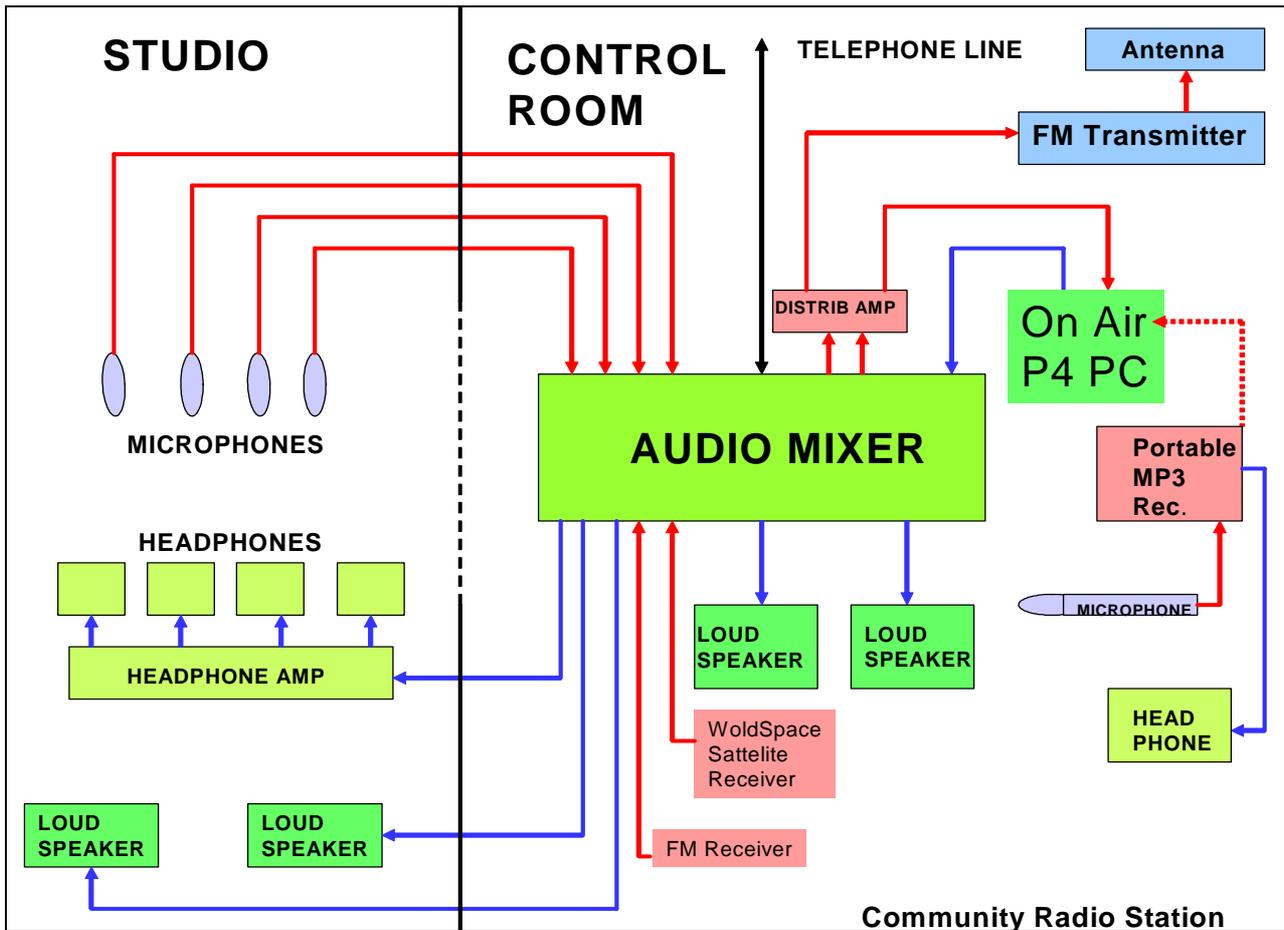
Fig. 20: Diagram of the Community Radio Station
