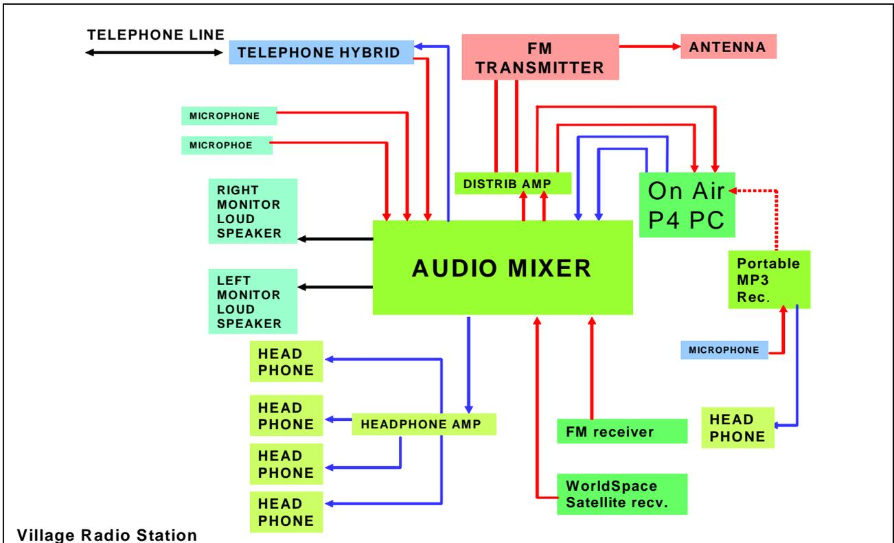
Fig. 15: Diagram of the Village Radio Station
