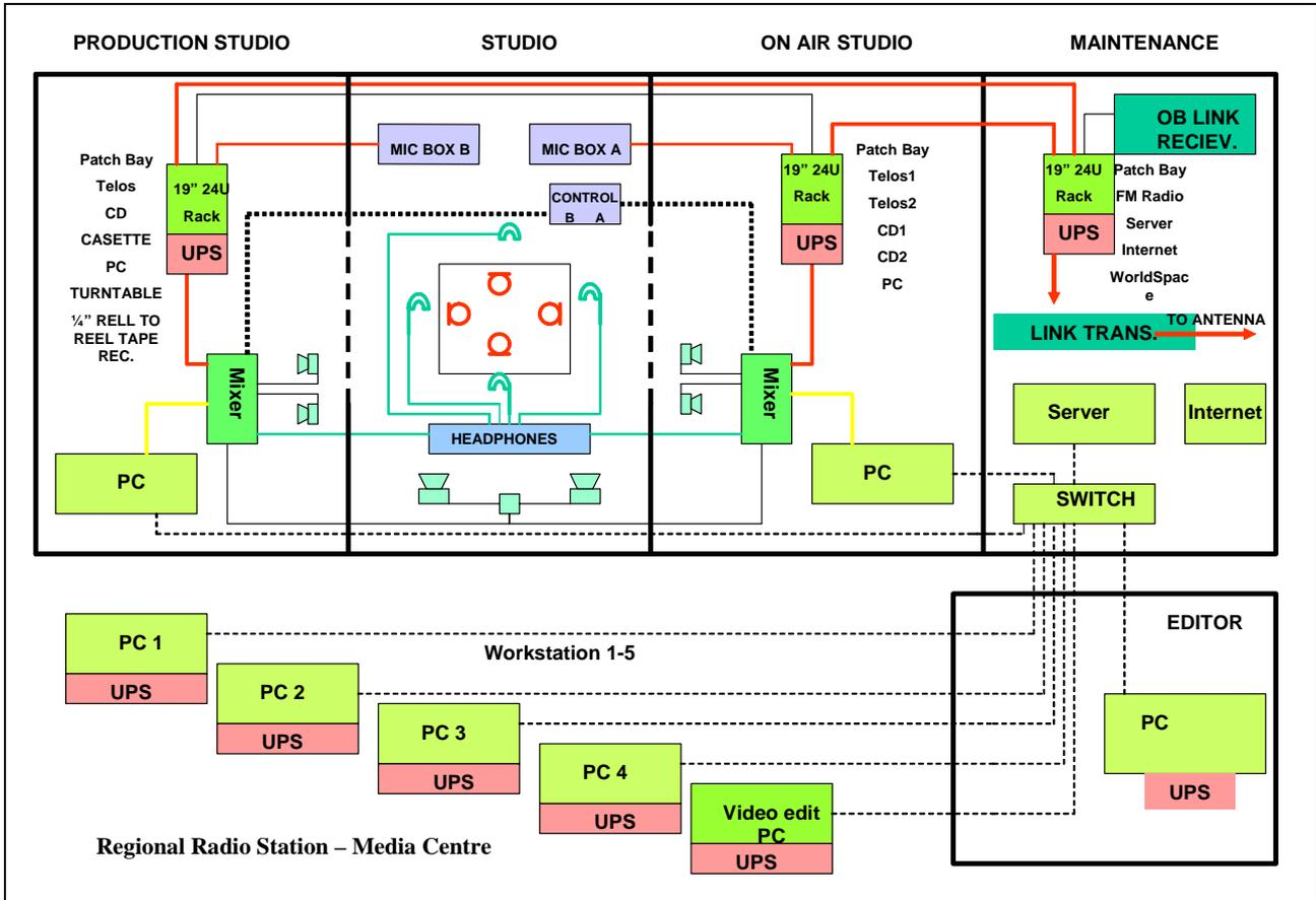
Fig. 21: Diagram of the Regional Radio Station
