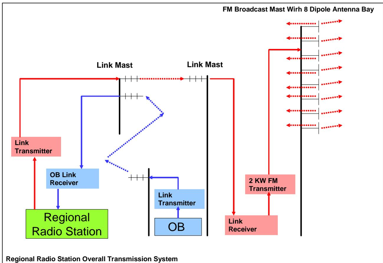
Fig. 28: Transmission system for the Regional Radio Station
