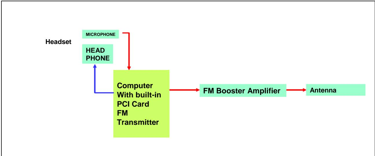
Fig.14: Diagram of the Micro Radio Station, example 2
